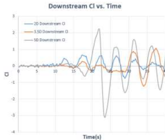
Figure 7. Lift coefficient time history of downstream cylinder
